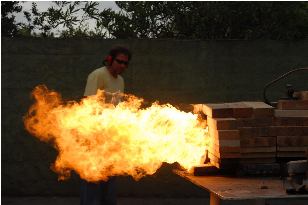
Fig.2: Operating conditions where the flame length exceeds the length of the combustion chamber [4].
